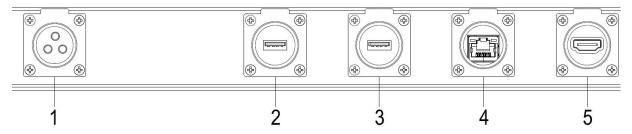
1. Power Socket 2. USB Port 3. USB Port 4.RJ45 Port(Ethernet) 5. HDMI Port **NOTE**: Please pull out the power plug before installing or disassembling the unit!
