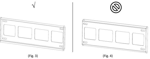
(Bracket should lay flush to wall, with raised portion facing out)
